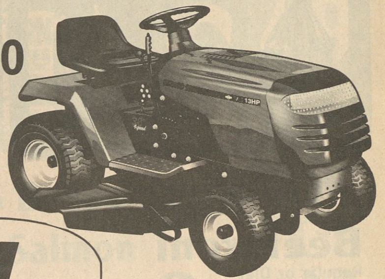
Wizard 38 in. 13.0 h.p. lawn tractor. 4-speed transaxle. Briggs & Stratton I/C quiet engine. Full light panel. 93-7134-5
